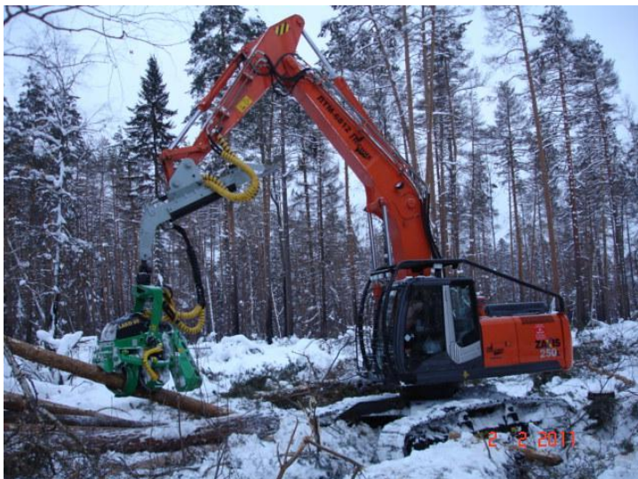
The TuLAKO 85.4 harvester head working in Russia with 25 ton excavator
