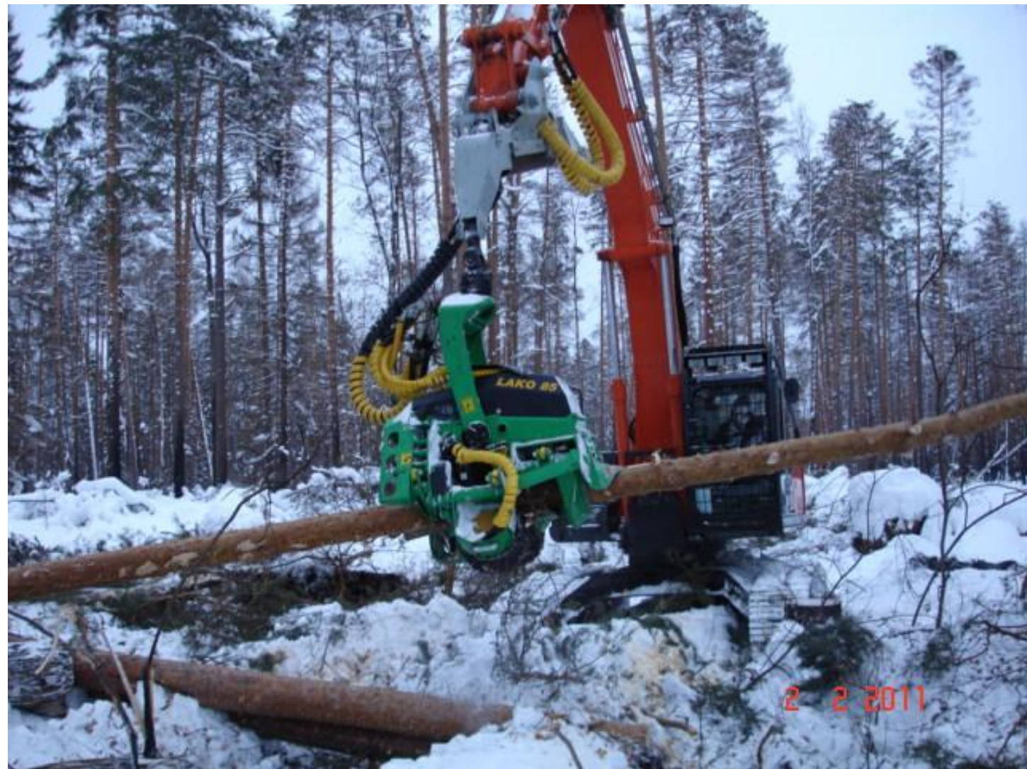
The TuLAKO 85.4 harvester head working in Russia with 25 ton excavator
