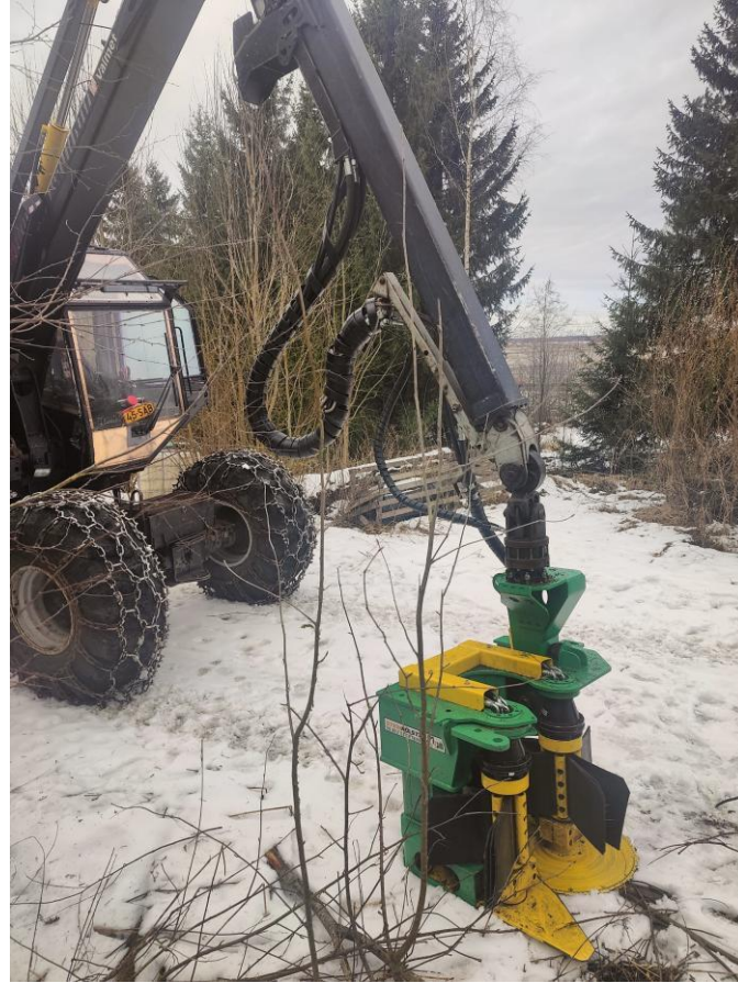
Second hand small scale forest machine can be utilized as a StemMaster's base machines
