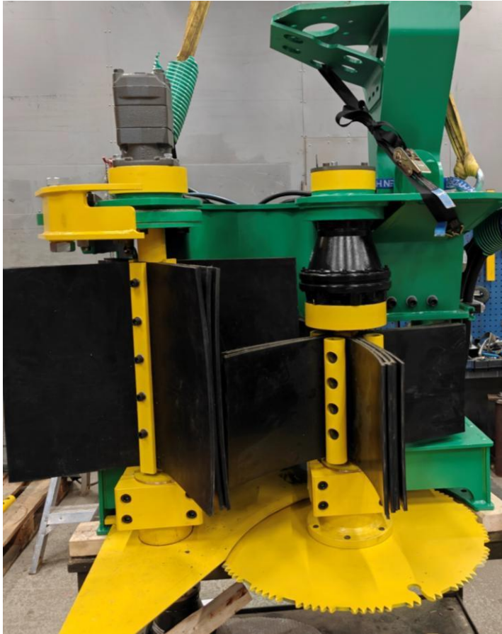
The continuously stem collecting system with an integrated cutting blade is the key principle
