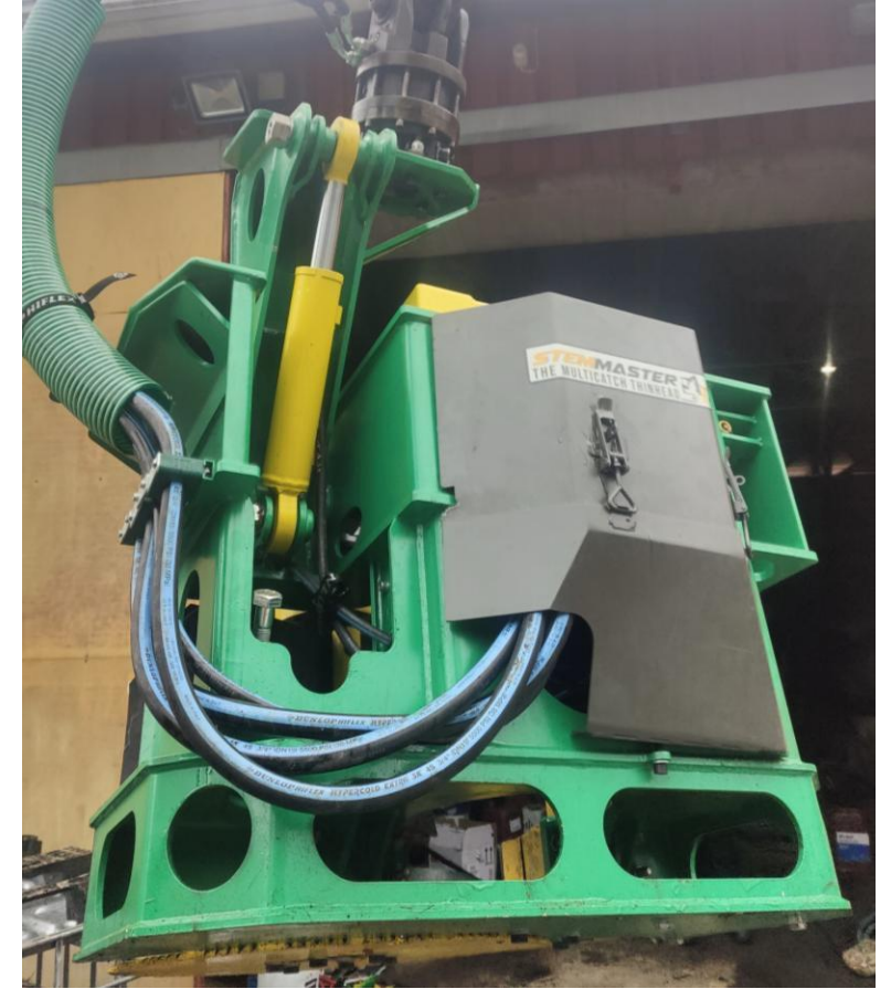
StemMaster bioenergy heads have a simple robust design with a modern hydraulic system
