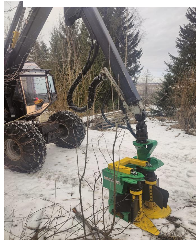
The diameter range or variation of the handled stems is from 1 cm up to 15cm with 250 head and up to 20cm with bigger capacity StemMaster 300.
