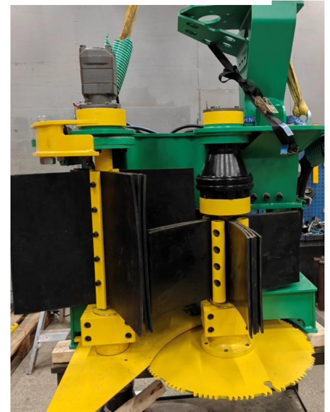
The diameter range or variation of the handled stems is from 1 cm up to 15cm with 250 head and up to 20cm with bigger capacity StemMaster 300.
