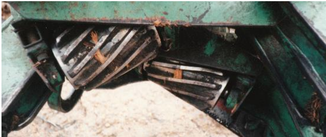
Grapple arm geometry LAKO harvester head with 4 motors / 4wd drive. The very first arm geometry solution
